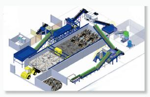
These processes enable the separation of high-purity plastic waste with low contaminant content, which is then used as raw material in Chemcycle's waste plastic recovery system.
